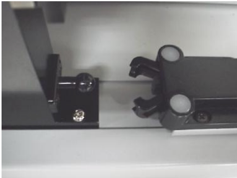
Figure 29: Ball Joint and Locking Mechanism
