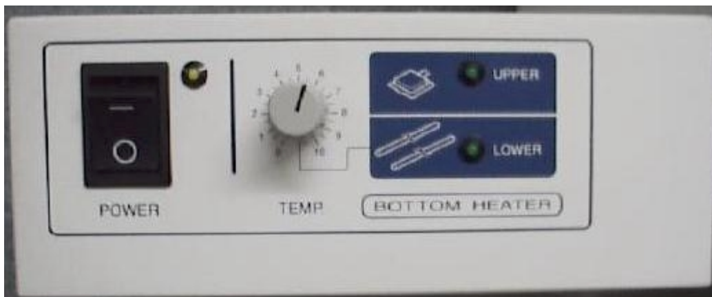
Figure 28: Switch Panel for the Movable Bottom Heater
