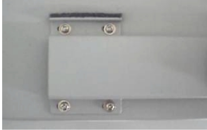
Figure 30: Locking Mechanism Mounting Bracket (Top View)
